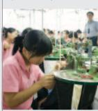
The garment parts are joined carefully to make a sweater. While joining the knitted parts with the same kind of thread, the seamstress checks for any skipped stitches and damage to the fabric.
