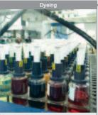
Several dye shades are mixed to achieve the prop er depth of color. To ensure products are dved the same hue, maintaining temperature and humid at the right levels in the dveing process is vital.
