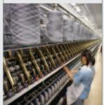
The yarn is then stretched out to about 20 times its length until it becomes a strand. To give the yarn a uniform thickness, it is essential to optimally maintain the high-speed, revolving spinning machines.
